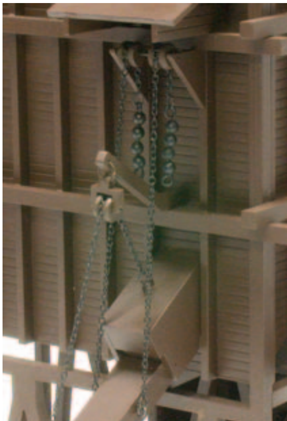
Metal chains with counterweights are owner-installed over functional plastic pulleys.
